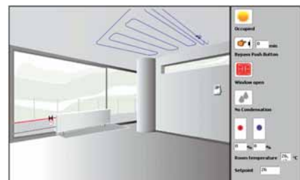
Heating with radiator, cooling with chilled ceiling
