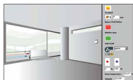
Heating/cooling with fan coil unit, electric reheat
